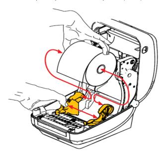
**Step 3** - Verify that the movable black mark sensor is aligned in the center default position. This is the standard operating position for media sensing. When the sensor is moved from the default label web (gap) sensing area, the printer will only detect black mark and die-cut notched media.
