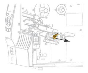
**Step 5** - From the media hanger (1), feed the media under the dancer assembly (2), through the media sensor (3), and under the printhead assembly (4). Slide the media back until it touches the inside back wall of the media sensor.
