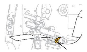
B) Rotate the printhead-open lever downward until it locks into place.
