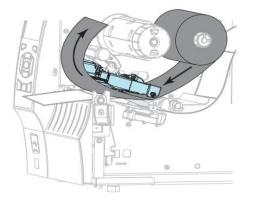
Step 5 - With the ribbon tracking as far back as it can under the printhead assembly, wrap the ribbon around the ribbon take-up spindle. Rotate the spindle several turns in the direction shown to tighten and align the ribbon.
