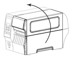
Step 2 - Open the printhead assembly by rotating the printhead-open lever.
